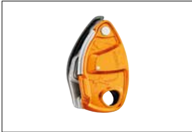
GRIGRI® + Belay device with assisted braking and anti-panic function, for a broad range of single rope diameters (8.5 to 11 mm). Choice of belay mode: top-rope or lead climbing.
