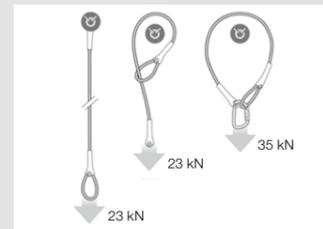
It offers several configurations for setting up an anchor: directly to an anchor point or around a suitable structure.
