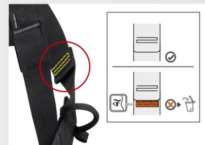
The sternal and dorsal attachment points are equipped with visual indicators: a red tag appears after a fall to indicate that the harness must be retired.
