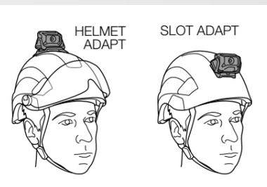
The headband allows ARIA headlamps to be worn on the head or around the neck. They can also be mounted on a helmet, with mounts available as accessories: HELMET ADAPT (compatible with a variety of helmet types) and SLOT ADAPT (for helmets with compatible slots).
