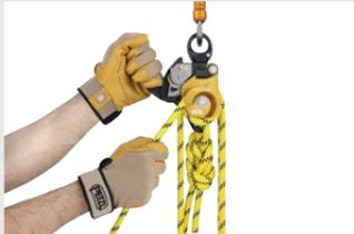
Release of the cam and passage of the rope through the brake integrated into the main moving side plate, allows comfortable and precise control when lowering.
