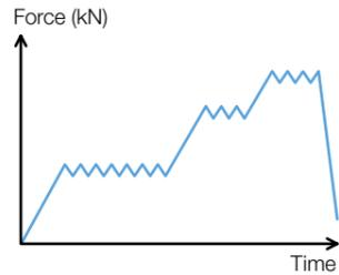
In the event of a fall, the tearing of the energy absorber webbing limits the impact force on the user. The lanyards are designed for users who weigh between 50 and 130 kg. The progressive tearing of the webbing reduces the deceleration on lightweight users.
