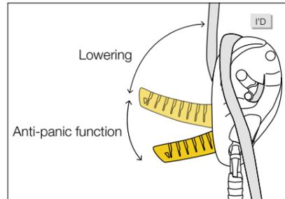
Designed for work at height, rope access, and technical rescue and evacuation, these devices are equipped with an anti-panic function and an anti-error catch, to reduce the risk of an accident due to user error. They are also compatible with auxiliary brakes, which help increase the friction for lowering heavy loads.
