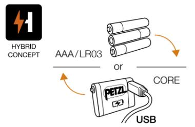
The HYBRID CONCEPT design allows the headlamps to function with standard AAA/LR03 batteries or with a CORE rechargeable battery. The headlamp automatically detects the energy source and optimizes lighting performance. With a rechargeable CORE battery, the lamp provides more brightness when it is turned on and throughout the duration of use.
