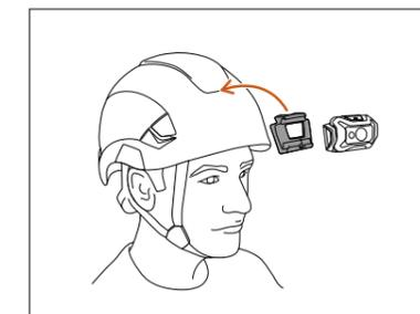
• On Petzl helmets, using specific mounting plates that are available as accessories
