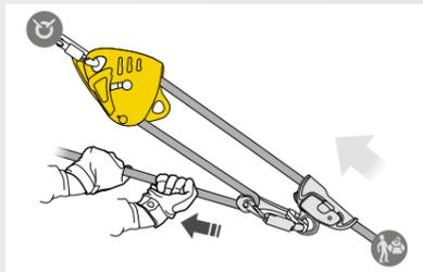
The integrated progress-capture pulley with very large diameter sheave mounted on sealed ball bearings rotates in only one direction for excellent hauling efficiency. The lower connection point can be used to create different types of haul systems.
