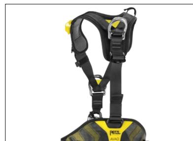
The AVAO BOD and AVAO BOD FAST full-body harnesses are equipped with a dorsal attachment point for connecting a fall-arrest system. In the event of a fall on this attachment point, a shorter adjustment of the length between the waistbelt and the leg loops means the load is taken up on the leg loops, allowing the user to remain suspended longer while awaiting rescue.
