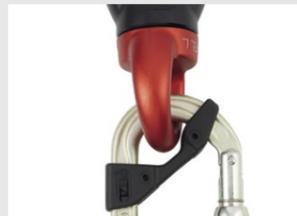
The oval, symmetrical shape allows the carabiner to be loaded in the optimal position when setting up anchors. Usage with the CAPTIV positioning bar promotes loading of the carabiner along the major axis, limits the risk of rotation, and keeps it attached to the device or lanyard.
