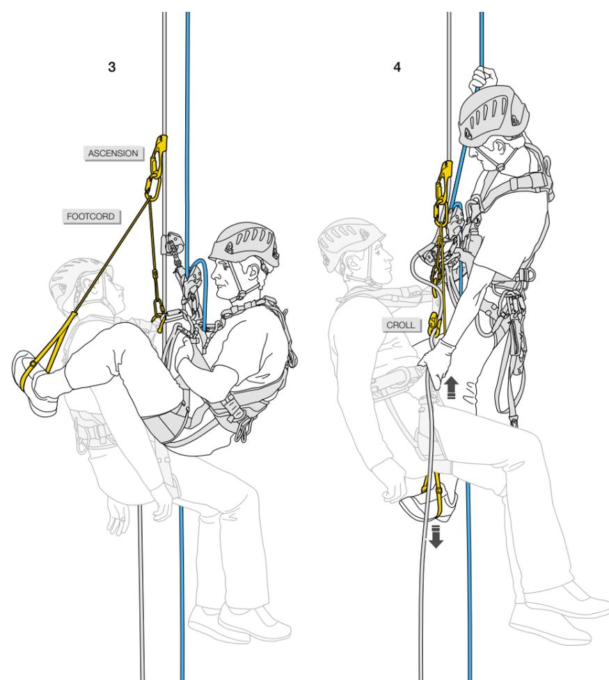
3. On the victim's rope, the rescuer installs a foot loop in counterbalance on the ASCENSION handled rope clamp.
