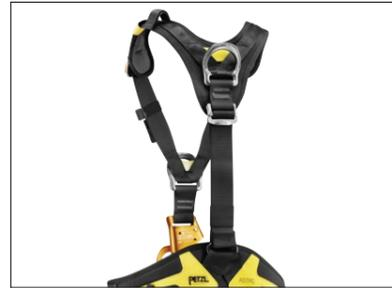
ASTRO BOD FAST full-body harnesses are equipped with a dorsal attachment point for attaching a fall-arrest system. In the event of a fall on this attachment point, a shorter adjustment of the length between the waistbelt and the leg loops means the load is taken up on the leg loops, allowing the user to remain suspended longer while awaiting rescue.
