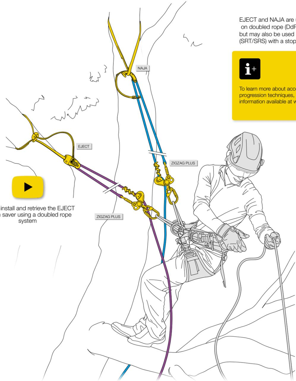
EJECT and NAJA are used here on doubled rope (DdRT/MRS), but may also be used on single rope (SRT/SRS) with a stopper knot.
