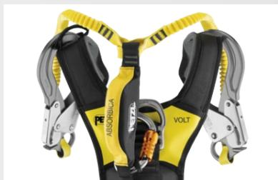
The harnesses have a parking system for the MGO connectors on fall-arrest lanyards on each shoulder strap. In the event of a fall, the system releases the MGO connectors and allows the absorber to be deployed.
