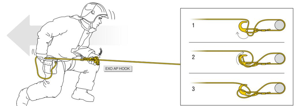
Going through a window while maintaining the anchor hook on the window sill. Locking the left leg against the interior wall to control the movement.
