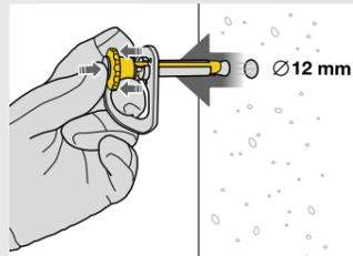
The anchor can be installed and removed for reuse very simply and rapidly, without tools.
