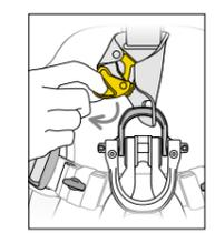
5. The rescuer, hanging on the RIG, removes the ASCENSION. They install a braking carabiner and accompany the victim to the ground.
