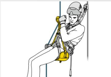
Self-braking descenders are versatile and can be used for both descents and short rope ascents.
