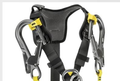
The harnesses have a parking system for fall-arrest lanyard connectors on each shoulder strap. In the event of a fall, the system releases the MGO connector and allows the absorber to be deployed.
